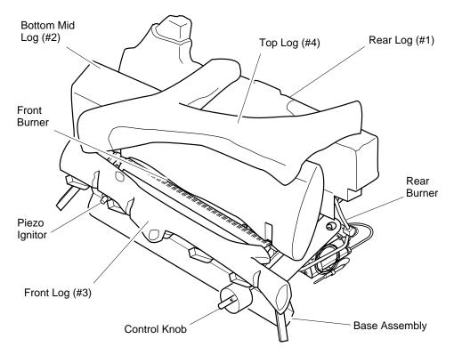
Figure 1 - Vent-Free Gas Log Heater
